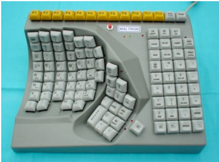
Maltron left-handed keyboard for one handed use
